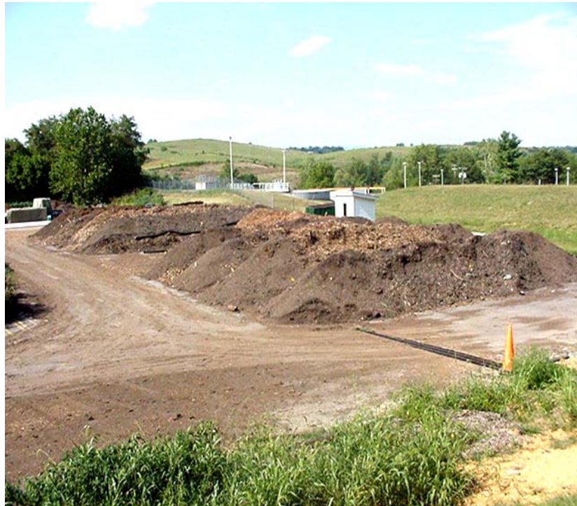
Figure 1. Aerated Static Pile
